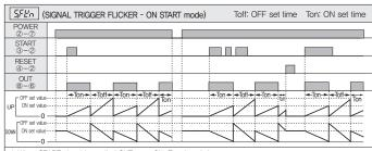
1. When START signal is applied OUT turns ON, Ton time timing starts 2. When the time value reaches the ON set value OUT turns OFF.
