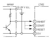
• Contactless input (when the sensor output is NPN open collector output)
