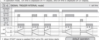
1, When START signal is applied OUT turns ON, and timing starts, 2. When time value reaches set value, OUT turns OFF, holds time value
