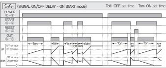
5, When RESET signal is cancelled, OUT turns ON and timing restarts if the START signal is applied
