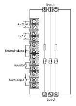
■ How to wire the input signal terminal
