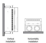
Product installing direction should be vertical direction. If you need to install this product as the horizontal direction due to the space problem or etc. please only use 50 % of the
