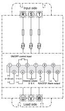
■ Input signal terminal connection diagram (Regular type / FND type)
